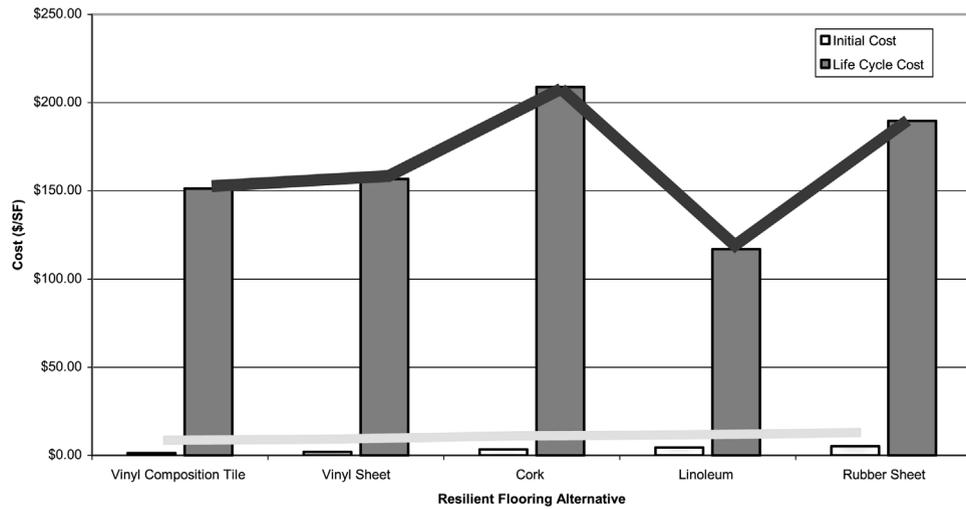
**Figure 12** Initial cost versus LCC – VCT and linoleum
