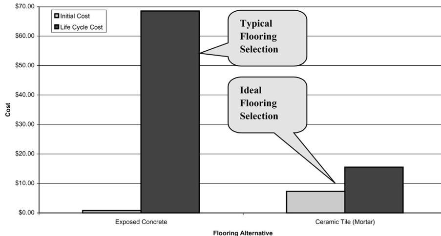
**Table II** Total cost comparison of a low initial cost option versus the low LCC option
