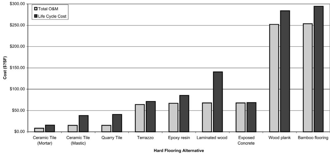
**Figure 8** Increasing O&M versus LCC
