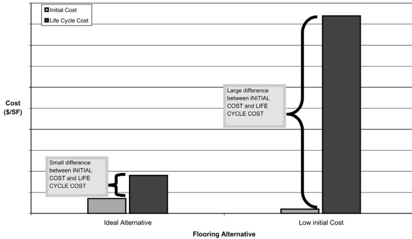
**Figure 4** Increasing initial cost versus LCC
