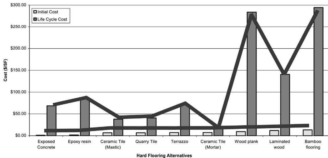
**Figure 6** Exposed concrete versus ceramic tile (mortar)
