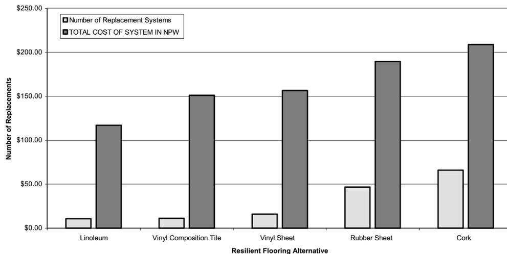
material, the fewer the replacements, the lower the total NPW of the alternative.
