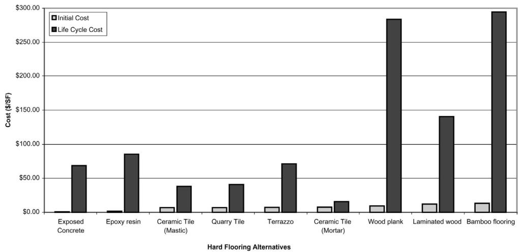
**Figure 5** Increasing initial cost versus LCC
